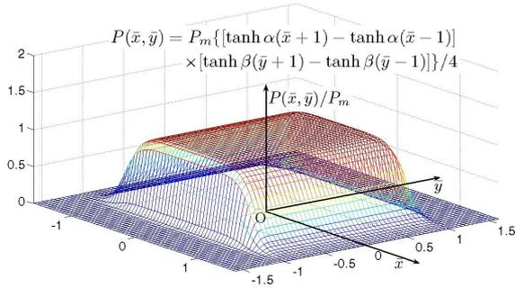
Figure 2: Pressure function  $P(x, y)$  of a cushion ( $\alpha=5, \beta=20$ ) in unitized variables:  $\bar{x} = 2x/B_p, \bar{y} = 2y/L_p$ .
