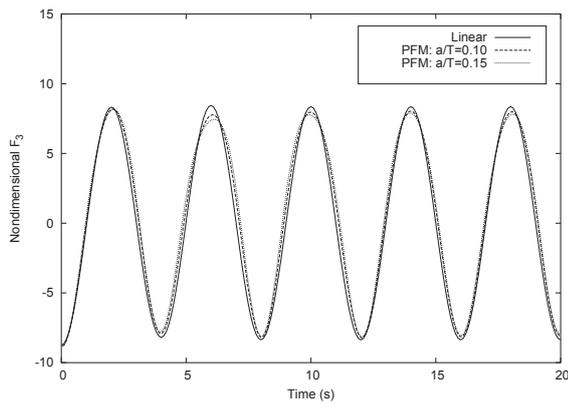
Figure 5: Heave forces at  $a/T=0.1$  and  $0.15$ ,  $\omega = \pi/2$
