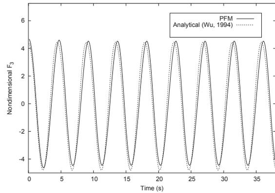
Figure 3: Heave force at  $\eta/R=1.0$  and  $kR=1.0$
