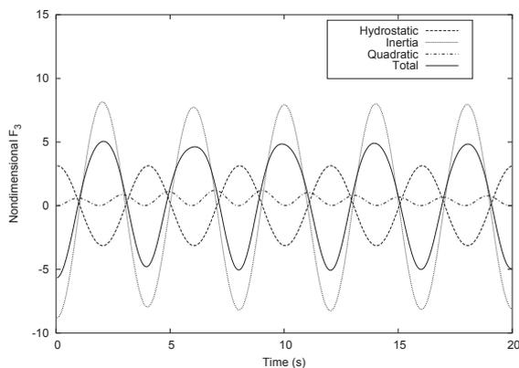
Figure 6: Heave force components at  $a/T = 0.1$ ,  $\omega = \pi/2$
