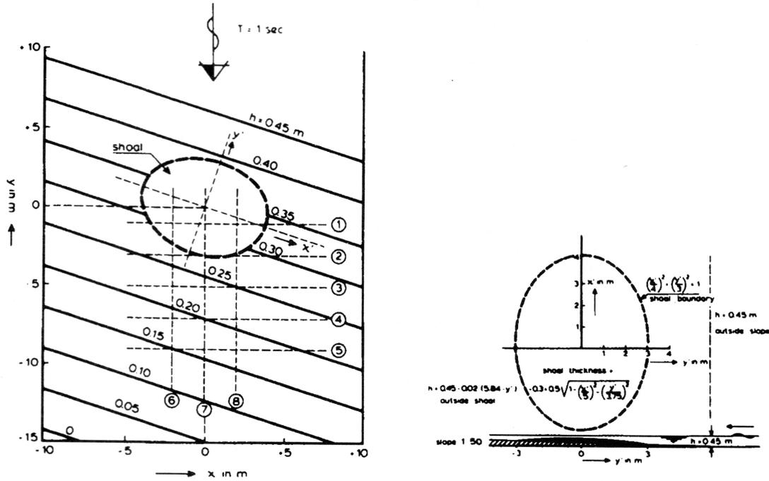
Figure 1: Setup of the elliptic shoal test case.
