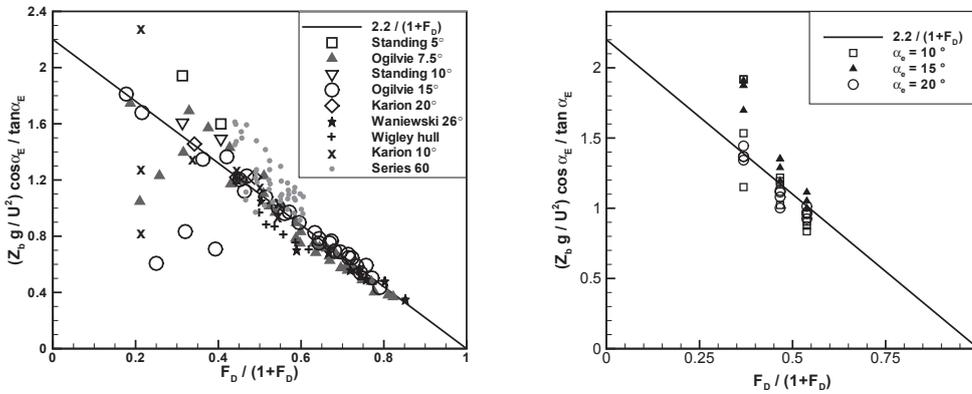
**Fig.1** Normalized bow-wave height  $(Z_b g / U^2) \cos \alpha_E / \tan \alpha_E$  for nine ship hulls (left) and a flat plate towed at speed  $U$ , draft  $D$ , incidence angle  $\alpha_E$  and flare angle  $\gamma$  (right). The straight line is the approximation  $2.2 / (1 + F_D)$  given by (1).
