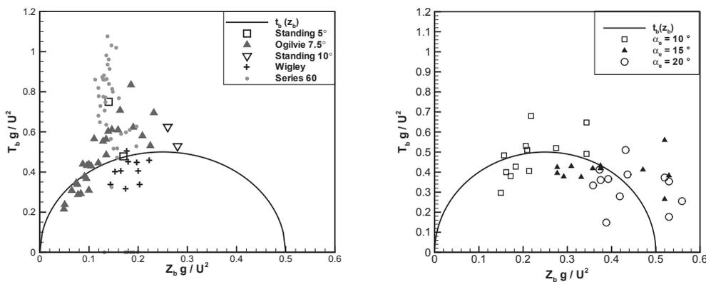
**Fig.3** Nondimensional distance  $t_b = T_b g / U^2$  between a ship stem and bow-wave crest for five ship hulls (left) and a flat plate towed at an incidence angle  $\alpha_E$  and a flare angle  $\gamma$  (right). The distance  $t_b$  is depicted as a function of the nondimensional wave height  $z_b = Z_b g / U^2$ , and the circle is the approximation  $t_b = \sqrt{2 z_b (1 - 2 z_b)}$  given by (3).
