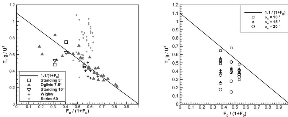
**Fig.2** Nondimensional distance  $t_b = T_b g / U^2$  between a ship stem and bow-wave crest for five ship hulls (left) and a flat plate towed at an incidence angle  $\alpha_E$  and a flare angle  $\gamma$  (right). The straight line is the approximation  $1.1 / (1 + F_D)$  given by (2).
