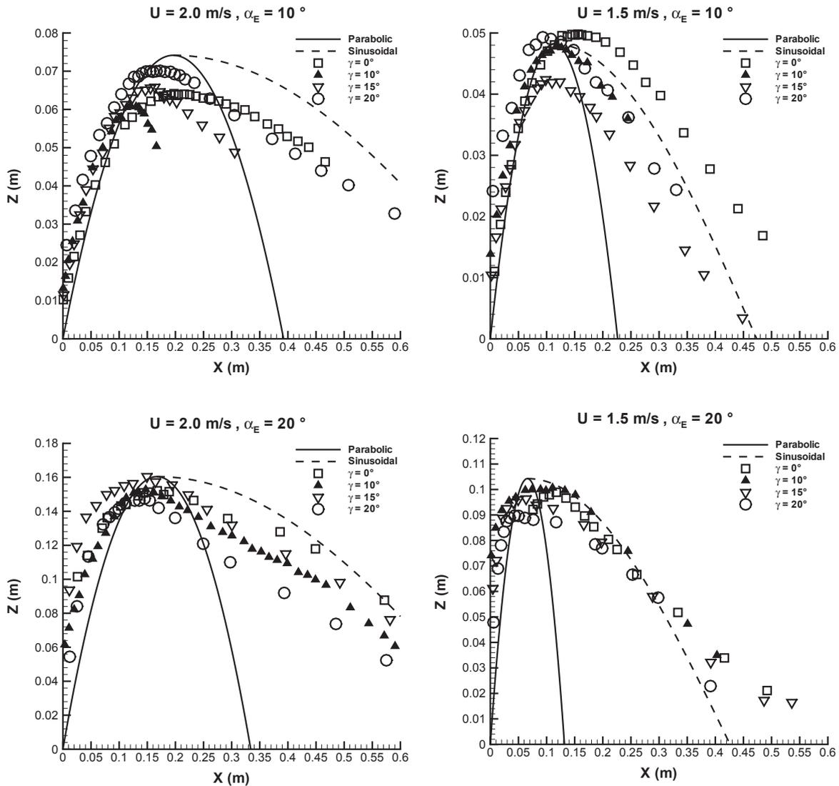
**Fig.4** Comparison of the simple analytical bow-wave approximation given by (5) and (1) with experimental measurements for a rectangular flat plate immersed at a depth  $D = 0.3\text{ m}$  and towed at flare angles  $\gamma = 0^\circ, 10^\circ, 15^\circ, 20^\circ$  and incidence angles  $\alpha_E = 10^\circ$  (top half) or  $\alpha_E = 20^\circ$  (bottom) with speeds  $U = 2\text{ m/s}$  (left side) or  $U = 1.5\text{ m/s}$  (right).
