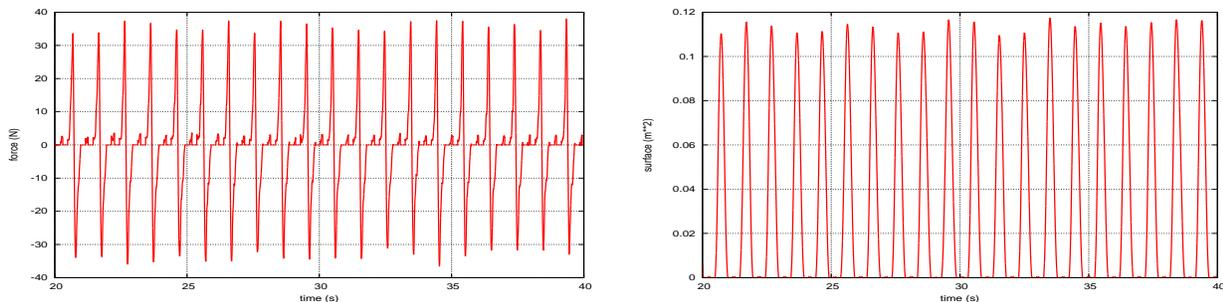
It is worth noticing that the positive and negative maxima of the force are of the same magnitude. This was also revealed by Barrholm (2001). These plots also show that the repeatability of each impact of standing wave crest is reasonable consistently with the repeatability of the measured wave kinematics. In order to check this point, the force is plotted in term of the wetted surface (figure below, on the left).
