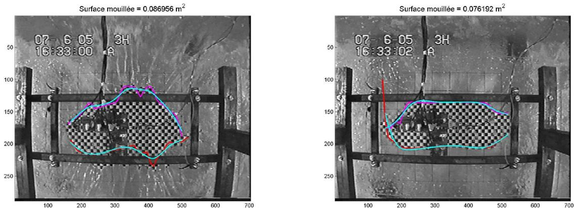
The duration of the measurements depend on the time during which the standing wave pattern is stable. As soon as the reflection on the wavemaker gets sensitive in the vicinity of the vertical reflecting plate, measurements stop.
