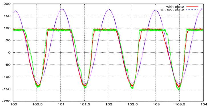
When the flat plate is hit, the wave gauges saturate at a threshold which corresponds to the airgap  $h$ . What is most noticeable is the larger slope of the ascending wave. This means that the local vertical velocity increases due to presence of the flat plate. This vertical velocity is calculated by a time differentiation of the wave elevation. This leads to a very irregular signal and a smoothing is necessary. The figure below shows a time sequence of the velocity variation.
