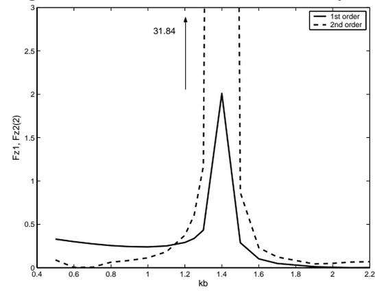
Fig. 8: Heave forces on the inner body,  $h_1/h=0.8$
