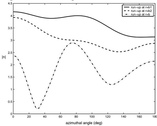
Fig. 3: Wave run-up for  $h_1/h=0.68$ ,  $kb=1.25$
