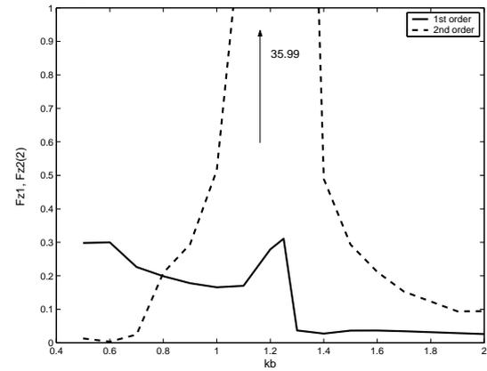
Fig. 6: Heave forces on the inner body,  $h_1/h=0.5$
