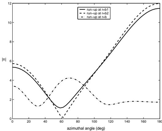
Fig. 4: Wave run-up for  $h_1/h=0.80$ ,  $kb=1.4$
