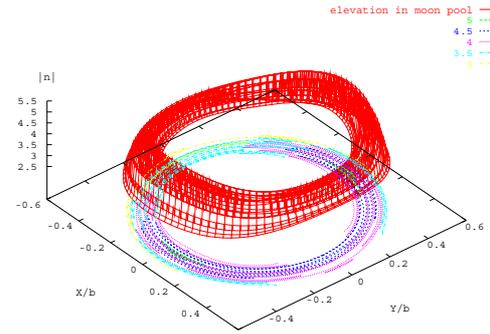
Fig. 5: Free surface elevation in the moonpool,  $h_1/h=0.68$ ,  $kb=1.25$
