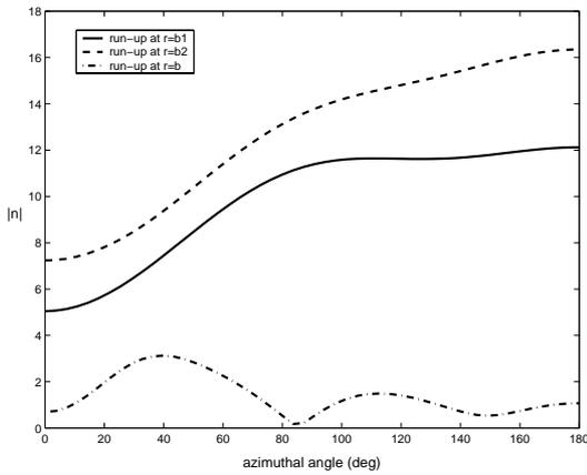
Fig. 2: Wave run-up for  $h_1/h=0.50$ ,  $kb=1.25$
