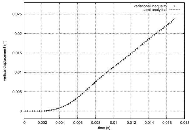
Figure 4: Vertical deflection with respect to time for the point situated at 50 cm of the centre
