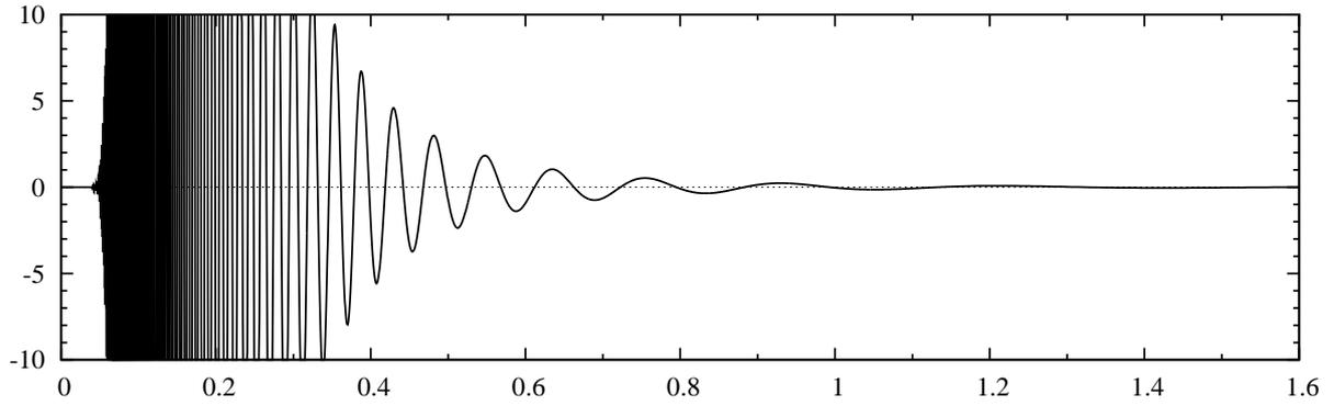
Figure 1: Potential function  $\Phi_t(h, z, t)$  at  $z = -1/1000$  and  $t = 10$  against  $h$  varying from 0 to  $8/5$ , obtained by taking only account of the fluid viscosity ( $\epsilon = 3.193e-7$ ) but without the surface tension ( $\sigma = 0$ ).
