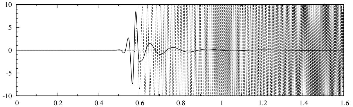
Figure 2: Gravity-dominant waves (solid line) and capillary-dominant waves (dashed line) of potential function  $\Phi_t(h, z, t)$  at  $z = -1/1000$  and  $t = 10$  against  $h$  varying from 0 to  $8/5$ , obtained by taking account of surface tension ( $\sigma=2.713e-3$ ) but without the fluid viscosity ( $\epsilon = 0$ ).
