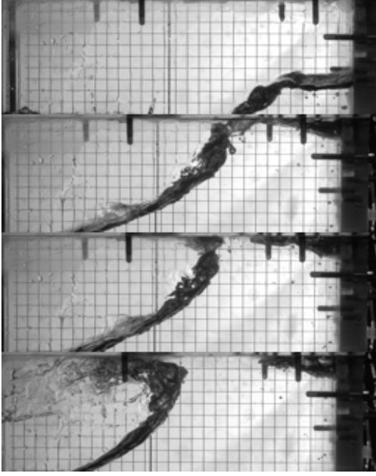
Figure 4: Pictures of impact with air cavity
