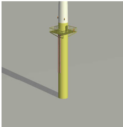
Figure 1 Monopile foundation for offshore wind turbine.
