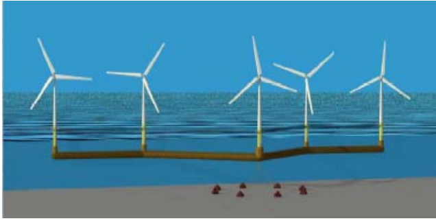
Figure 3. Multi-turbine floater, Hendrikson, 2003
