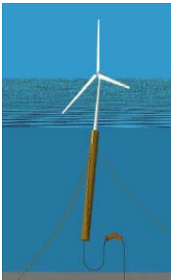
Figure 5. Spar foundation, Henderson, 2003
