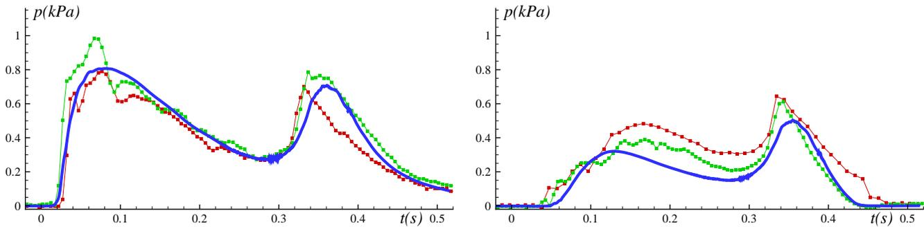
Figure 7: Pressure evolution at the wall locations  $0.24f$  (left) and  $0.64f$  (right) above the deck, with  $f = 0.05$  m the ship freeboard. The water-on-deck has been caused by prescribed regular incident waves  $\lambda = 40f$  long and with a crest-to-trough height  $H = 0.08\lambda$ . Lines with symbols: experiments by Greco (2001), two runs are shown for each pressure sensor. Solid lines: DDDC results. Here  $t = 0$  s the time instant of the initial water-wall impact.
