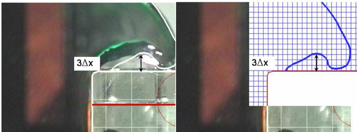
Figure 4: First water-on-deck caused by prescribed regular incident waves with  $\lambda = 40f$ ,  $H = 0.08\lambda$  and  $f = 0.05$  m. Initial plunging phase. The shown grid represents the numerical mesh used in the DDDC simulations.  $\Delta x = \Delta z \simeq 0.04f$ .
