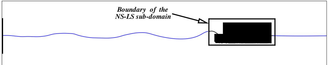
Figure 1: Domain-decomposition strategy applied to the water-on-deck problem. The incoming waves are generated by a flap wavemaker on the left and interact with a ship-like structure. This case refers to the model tests discussed in Greco (2001). The solid box delimits the fluid region described by the NS-LS method. The surrounding sub-domain is solved by the BEM. The horizontal size of the NS-LS region is about 0.08 times the domain extension.
