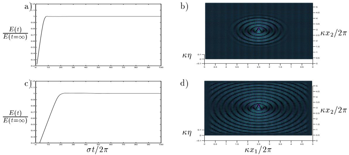
Figure 2: Relative energy evolution and free surface profile at  $\sigma t/2\pi = 100$  for two different dampers: a-b) circular damper, c-d) squared damper.
