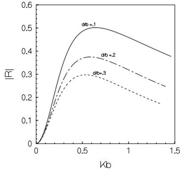
Fig.1: Reflection coeff. vs wave number,  $a/b=0.5, \alpha=0^\circ, \eta=180^\circ, s=0.2$
