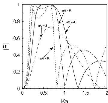
Fig.4: Reflection coefficient vs wave no.,  $b/d=1, \alpha=90^\circ, \beta=90^\circ, s=0$
