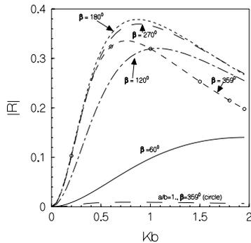
Fig. 2: Reflection coefficient vs wave number,  $a/d = 0.2, b/d = 0.8, \alpha = 0^\circ$
