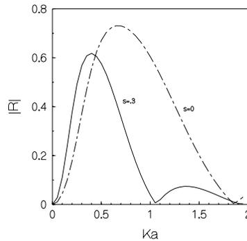
Fig.3: Reflection coeff. vs wave number,  $a/d=0.2, b/d=0.1, \alpha=-90^\circ, \beta=90^\circ$
