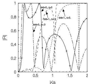
Fig.5: Reflection coeff. vs wave number,  $a/d=10, \alpha=90^\circ, \beta=90^\circ$
