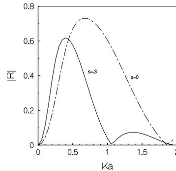
Fig.3: Reflection coeff. vs wave number,  $a/d=2, b/d=0.1, \alpha=-90^\circ, \beta=90^\circ$
