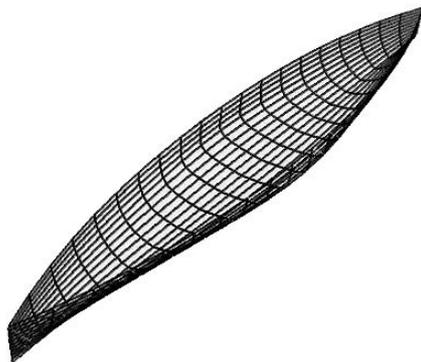
Fig.3 Boundary panels on the ship hull
