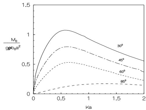
Fig. 4: Amplitude of moment per unit width vs wave number  $d/h=0.3, a/h=0.3$
