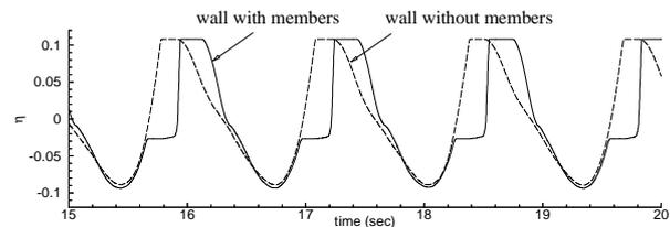
Figure 7. Surface elevation at two corners; the same tank with Figure 2; 80% filling,  $T_4=1.30\text{sec}$ ,  $A_4=4\text{deg}$ .
