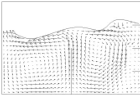
(a) Computed velocity vectors and elevation
