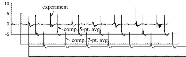
Figure 4. Pressure time-histories on tank top; the same tank with Figure 1, 70% filling,  $T_1=0.98\text{sec}$ ,  $A_1=0.038\text{m}$ ,  $30 \times 1 \times 20$  meshes,  $H = 0.5\Delta z$
