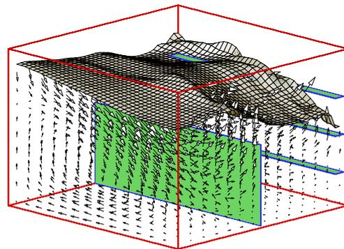
Figure 6. Instantaneous wave profile and velocity vectors in a 3-D tank; the same tank with Figure 2,  $B=0.8\text{m}$ ,  $T_4=T_5=1.30\text{sec}$ ,  $A_4=A_5=4\text{deg.}$ ,  $40 \times 40 \times 30$  meshes
