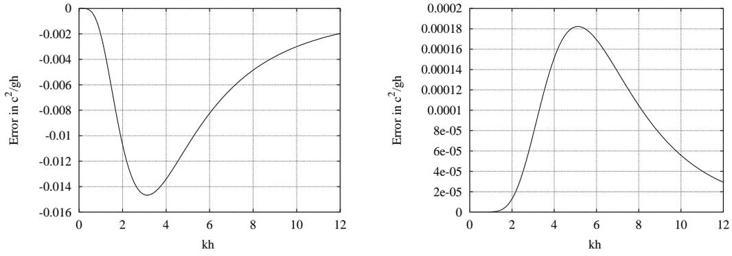
Figure 1: Relative errors in dispersion for Fourier-Boussinesq Padé(4,1) and Padé(8,2) methods.
