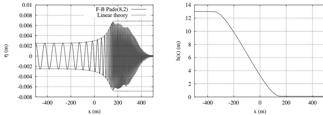
Figure 3: Linear shoaling for a wave of period  $T = 8$  s over the bottom shown. A wavemaker generates the waves from the left boundary and a sponge layer absorbs them at the right boundary.
