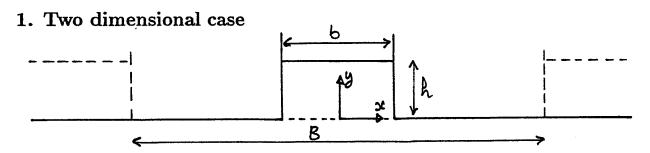
Let us first assume the beam of the barge to be infinite so that the geometry looks as sketched above. The fluid domain can be decomposed into two subdomains, by introducing a ficticious bottom to the moonpool: inside the moonpool, and the infinite half-plane y < 0.
