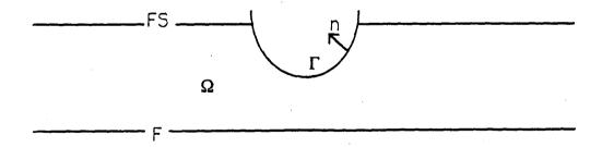
We study "the linearized steady-state problem", i.e., the periodic motion of the body subjected to a sinusoidal incident wave of frequency  $\omega$ . We want to determine the scattered potential  $\Phi$  as well as the motions of the body (C), characterized by the three components of a vector  $s = (s_1, s_2, s_3)$  (2 translations, one rotation).
