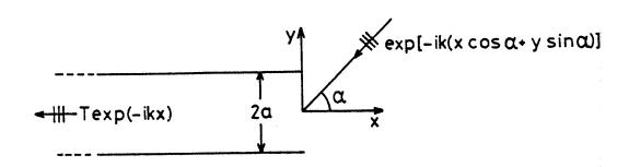
To determine T it is sufficient to consider that part of the solution that is symmetric in y. The symmetric part of the incident wave potential is
