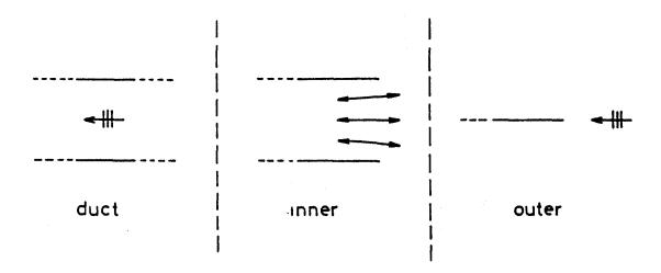
In the outer region the boundary condition on the breakwaters may be transferred onto y = 0 by Taylor expansion. Put  $a = \varepsilon a_1$  then
