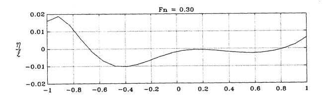
Fig. 1. Hull side wave profiles of WIGLEY
