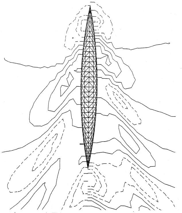
Computed wave pattern for Wigley parabolic hull. Broken lines are crests, full lines are troughs. The lines are  $0.05 \cdot U^2/2g$  apart.
