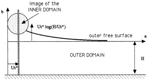
INNER AND OUTER DOMAIN FOR THE IMPULSIVELY PUSHED WAVEMAKER (SCHEMATIC)
