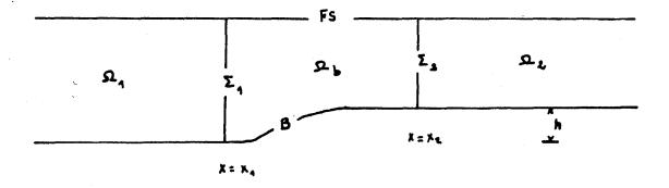
The dimensionless equations for the perturbation of the stream function  $\psi$  and for  $\eta$  the perturbation of the linearized free surface are given by the problem (P) : Find  $\psi$  fulfilling :
