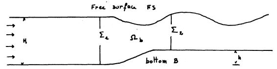
We consider an incompressible perfect fluid flow irrotational at infinity on an irregular bottom. The bottom irregularities have a compact support. The problem can be formulated in stream function or in potential function.
